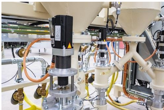
AKM servomotors by KOLLMORGEN with single cable connection technology in the Roxor shot-peening system (left). Shot (steel balls) for surface compaction (right).
